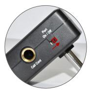
Lastly, make sure your coiled connector lead is correctly inserted into the bottom of the Jack.
