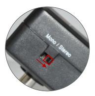
If it has 1 ring, it is mono (ensure the switch is at 'Mono'); as below example shows.
